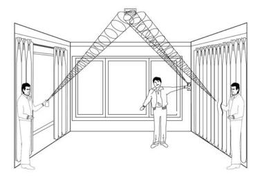
G. Press the handheld tester button labeled "Single." The expected and proper results are:
