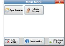
To return to the main screen press the EXIT MENU button or press the red close button on the top right of the screen.
