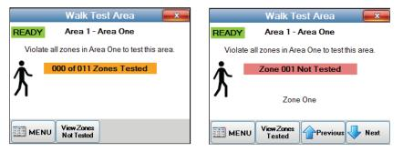
Navigator provides a quick and easy means of walk testing zones without distrurbing your neighbors. This Walk Test option DOES NOT cause any alarm or trouble reports to be transmitted to a Central Station.
