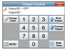
NOTE: Direct number entry is the only way to gain access to a hidden Output. The Next and Prevous buttons skip over hiddent Outputs.
