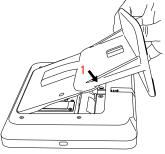
Locate the SmartMount table stand and insert the hooks into the back of the panel, then swing down and press into place.
