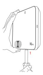
1. With a small phillips screwdriver, screw in the locking screw from the bottom of the panel to secure it to the wall.
