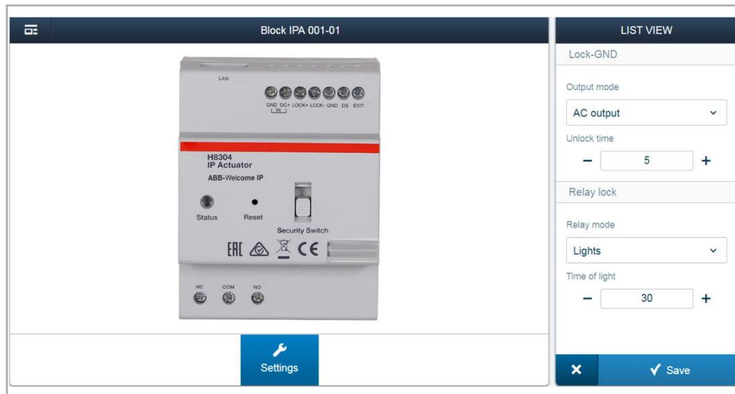
**(2) Set the trusted devices for the IP actuator**
