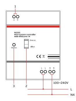
Serves as the brains and primary source of power of the door entry systems and manages communication between all components – outdoor stations, indoor stations, guard units, and other system components. It can also serve as auxiliary BUS power supply.
