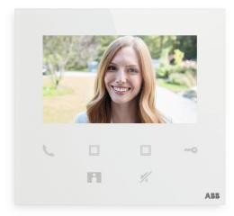
Video indoor station used to initiate and receive communication with outdoor stations, guard stations, and indoor stations. It is easy to install requiring only a single pair of non-polarized wires and connects to local Wi-Fi Signal to provide up to 8 App seats. It can be surface or table mounted.
