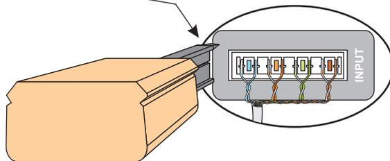
Connect any of the telephone outputs to wall plates in each room (see diagram).
