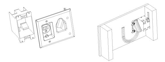
Once you have wired the receptacle, begin by inserting receptacle portion of the plate into the retrofit work box. Once the entire recessed plate is flush to the wall, using the two white screws supplied, screw the receptacle portion of the plate to the work box.
