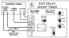
Provides an exit delay to an otherwise instant alarm loop. The ELK-960 is triggered by the control's Armed output. The door contact is then shunted by the relay contacts. After the user has exited and the delay time has expired, the door contact is restored into the loop.
