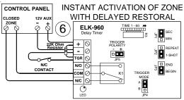
When contact opens, relay is turned on which causes instant zone violation. Contact reclosure will cancel trigger applied by resistor. Delay starts when contact closes. Relay turns off and zone restores after delay time expires.
