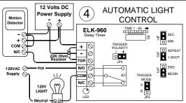
For turning on an interior or exterior light with a motion detector. When motion is detected, the ELK-960 is triggered and the light is turned on. The amount of time the light remains on after the detector resets is adjustable. Delay time will automatically restart each time the motion detector activates.
