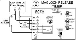
Used to extend the release time of an access control device or to manually activate a door **maglock** release device. The trigger is activated by a contact closure or a N/O pushbutton and the door maglock remains released (door open) after the button is released for the delay time set up in the ELK-960.
