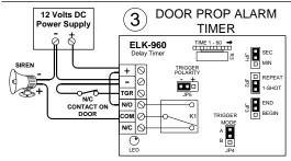
Delay is started when the door is opened. If the door remains opened after the time delay has expired the relay will turn on and remain on until the door is closed. If the door is closed before the time delay expires the ELK-960 is reset awaiting another input from the door contact.
