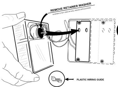
A) TWO ITEMS INCLUDED WITH THE STROBE KIT ARE NOT USED WITH A STAND-ALONE WALL MOUNT INSTALLATION:
