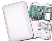
ELK-M1XEP Ethernet Interface For IP based lighting systems from Insteon/ Universal Devices
