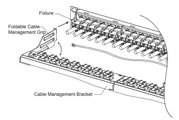
5. Fix the solid cables to the cable fixture hole using cable ties.
