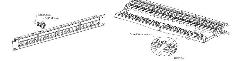
RJ45 modules are installed.
