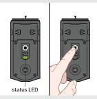
The latch bolt will retract and extend on its own to learn the orientation of the door. Did the Status LED turn green or red?
