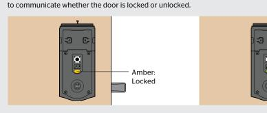
If the Status LED shows the opposite color to the latch bolt position, flip switch #4.
