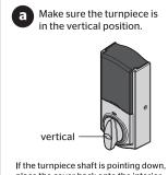
If the turnpiece shaft is pointing down, place the cover back onto the interior assembly and rotate the turnpiece until you hear it click. You may need to apply some force. Once the turnpiece shaft is correctly oriented, remove the cover again.
