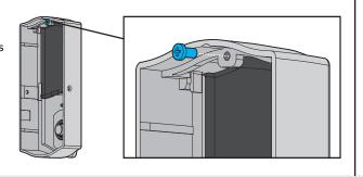
When the window is unlocked, you can slide up the window to access the battery pack and programming buttons.
