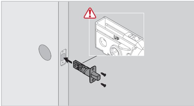
**D The turnpiece is upside down, or it cannot rotate to a vertical position.**
