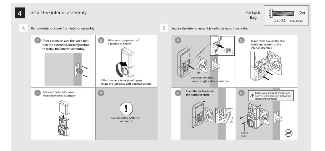
Install interior cover for the interior assembly.
