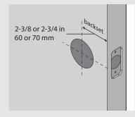
Measure to confirm that the hole in the door edge is 1 in (25 mm).
