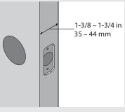
Note: Please contact customer service if door thickness exceeds 1-3/4 in for a thick door kit.
