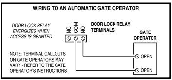
System Input Wiring
