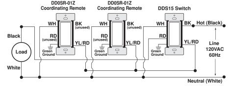
NOTE: The DDS15 switch must be installed in a wall box that has a Load connection. The DD0SR-01Z coordinating remotes must be installed in a wall box with a Neutral connection.
