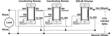
NOTE: The DD0SR-01Z coordinating remotes must be installed in a wall box with a Neutral connection. NOTE: "BK" and "RD" terminals on coordinating remotes are unused. Tighten screws.
