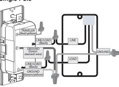
3-Way NOTE: To control the load from the 3-way switch, toggle once to turn the load ON and twice to turn the load OFF.
