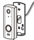
**4** Connect the power source to the IVPC-DS. If necessary, use the bypass cable (included) for the connection.
