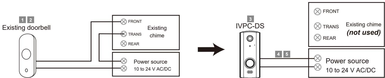
**1** Turn off power. Disconnect all wires from the existing chime.
