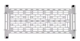
The On-Q mounting plate, AC1050, is constructed of WiFi transparent ABS plastic and is designed to securely mount a variety of 3rd party deives into the On-Q plastic structured wiring enclosures. The mounting plate can be mounted vertically or horizontally and include (4) plungers and grommets along with velcro strapping for devices to be safely secured inside the enclosure without compromising wireless performance.
