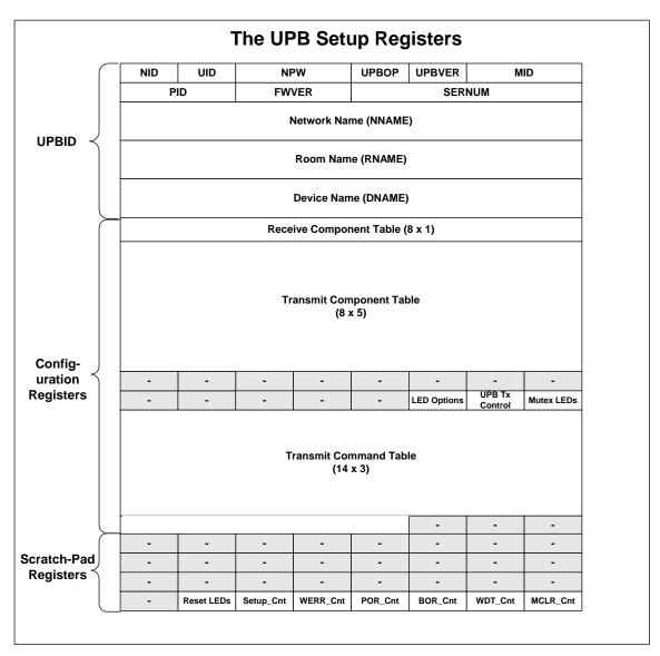
Figure 2: The WMC8 UPB Setup Registers
