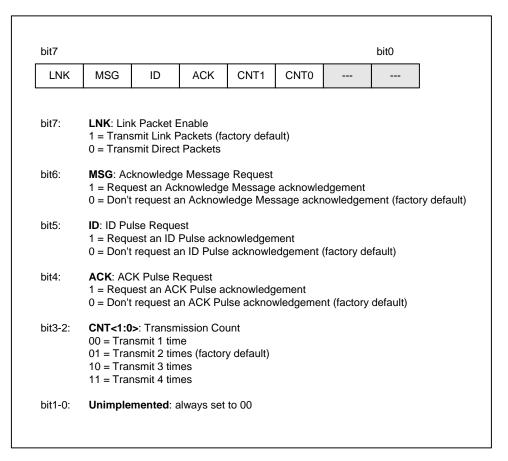
Figure 4: The UPB Transmit Control Register
