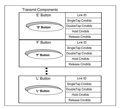
Figure 3: 8-Button Controller's Transmit Components
