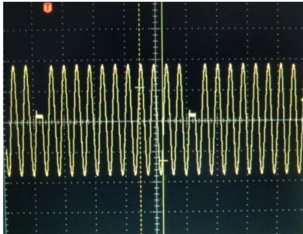
It is impossible for this signal method to go backwards into the circuits of the building. The relay load line goes **ONLY** to the fixtures on the load line (red wire). It is impossible for anything in the building to attenuate the missing  $\frac{1}{2}$  cycles. When the relay is open it is OPEN. It is only a simple mechanical power relay. The same relay type that has been used in all occupancy sensors and relay type switches for the past 20 years.
