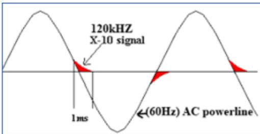
The oldest power line signal protocol is X10 and uses the 60hz sine wave of the power line as a carrier for the insertion of a message at selected points. The image on the left shows this graphically.
