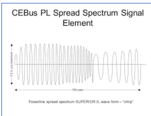
Another method that was developed as an attempt for X10 to address attenuation and noise issues was CEbus spread-spectrum.
