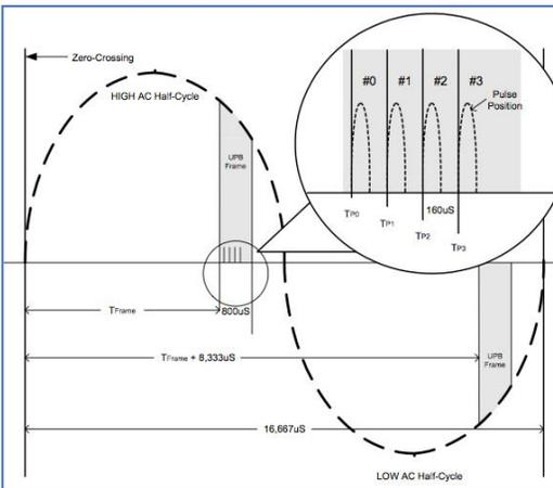
A modern method that uses the power line, developed by PCS, is called UPB and uses Pulse Position Modulation. UPB messages transmit digitally encoded information over the power line as a series of precisely timed electrical pulses.
