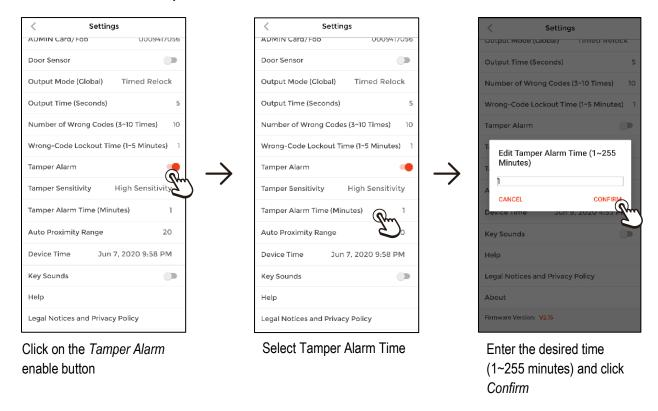
**NOTE:** The tamper alarm will sound an internal buzzer and will output to an external alarm if connected. It will continue until the time expires or until the ADMIN disables the tamper alarm in the app. The tamper alarm can be immediately re-enabled for continued protection.
