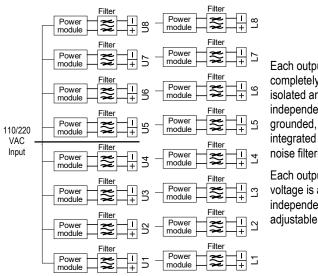
Each output is completely isolated and independently grounded, with noise filtering.
