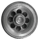
clear valve no blockage
