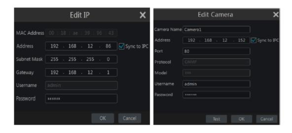
Click to edit the added camera as shown on the above right. Input the new camera name, IP address, port, username and the password of the camera. You can click "Test" to test the effectiveness of the input information. Click "OK" to save the settings. You can change the IP camera name only when the added camera is online. Click "Next" to continue.
