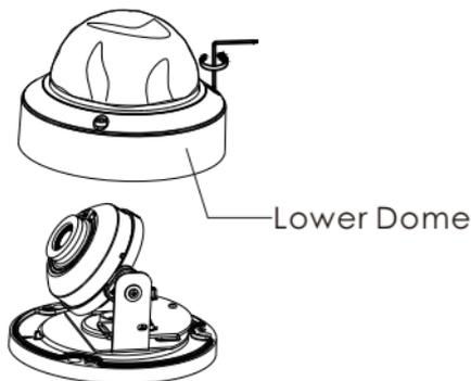
③ Route and connect the cables. Then secure the camera to the ceiling or wall with the screws provided.
