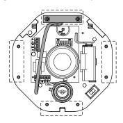
11. Install reed magnet, mark with pencil, drill, install using plastic anchor, drill 3/16" (4.5mm). Install into wood or steel: drill 1/8" (3mm). Mount with (2) M3.5 x 32mm screws.
