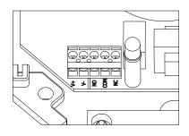
7. Test – place magnet next to reed, turn key switch on, separate magnet from reed
