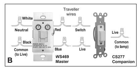
The WS469 is designed to control Lighting and Appliances up to 10Amp 1000 Watts. The switch can replace a single switch, however, it can also be used where two switches control the same light (3-way). In this case a Companion Switch (CS277) is required and is sold separately. A push-button is provided on each switch for local on/off control.
